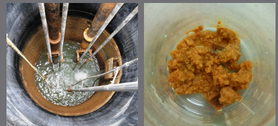
Figure 2. Images of the transfer well (left) and scale sample removed from the second stage vessel (right). A sample of the orange granular material from the second stage vessel was collected and returned to Avista lab for analysis. The sample was analyzed and identified as calcium sulfate scale combined with iron. (Figure 2)
