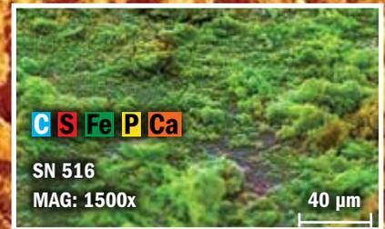
concern when the plant was designed, but as water levels decreased, the wells closest to each other competed for available groundwater. Operations staff noticed “rumbling” and “shaking” when the affected wells were placed online, especially when a higher demand was placed on the wells. In both instances, cascading of the wells entrapped air, causing iron oxidation and a resulting cartridge-filter and RO-fouling event.
