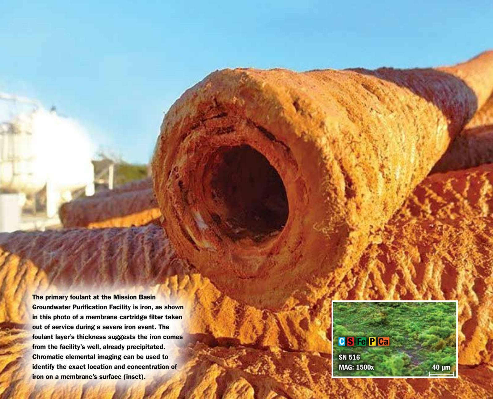
The primary foulant at the Mission Basin Groundwater Purification Facility is iron, as shown in this photo of a membrane cartridge filter taken out of service during a severe iron event. The foulant layer's thickness suggests the iron comes from the facility's well, already precipitated. Chromatic elemental imaging can be used to identify the exact location and concentration of iron on a membrane's surface (inset).
